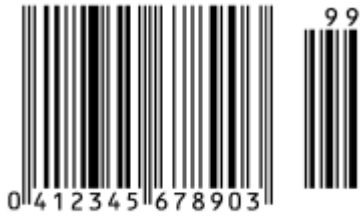
EAN + 2 Digit Supplemental (encoding 041234567890, supplemental = 99)
