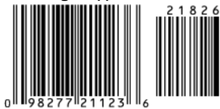
UPC A + Five-digit Supplemental (encoding 09827721123, supplemental = 21826)
