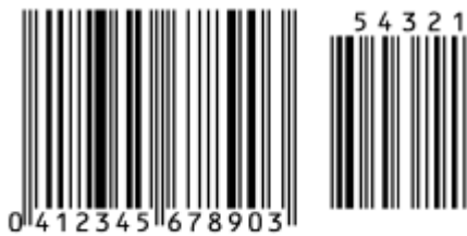
EAN + 5 Digit Supplemental (encoding 041234567890, supplemental = 54321)
