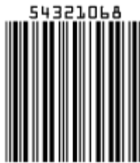
Interleaved 2-of-5 (encoding 54321068)
